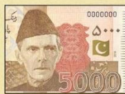
7 Intaglio Printing Quaid-e-Azam's portrait, numeral 5000 and the lines at left & right side of the note are printed by intaglio process. One can easily feel the raised printing by touching the note.
