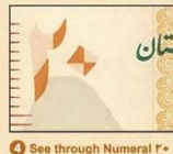
4 See through Numeral 20 The numeral 20 printed in Urdu with one half of the digit on one side and the other half on the other side can be seen as a complete digit when held against the light.
