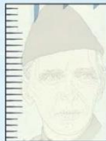
1 Portrait Watermark When the note is held against the light, an image of Quaid-e-Azam can be seen.
